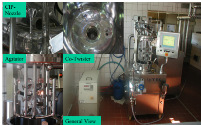
Fig. 1: Processing facility - Symex CML 30
